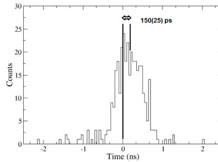
**Figure 2:** A time distribution spectrum showing the time difference between the centroid of the forward time spectrum and the prompt position of gamma rays feeding and de-exciting the level of interest. Five gates were used to select the 992- and 1609-keV transitions. After using data from both TAC settings,  $\sim 350$  counts were obtained in 10 days. Preliminary analysis of this time difference indicates a half-life of  $\sim 150$  ps for the  $i_{13/2}$  level.
