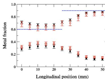
**Figure 2.** Atomic fractions of indium (circles) and zinc (squares) measured by LIBS (empty red symbols) and by EDS (filled black symbols). The dashed lines represent the In/(In+Zn) fractions of the targets used for thin film synthesis by C-PLD.
