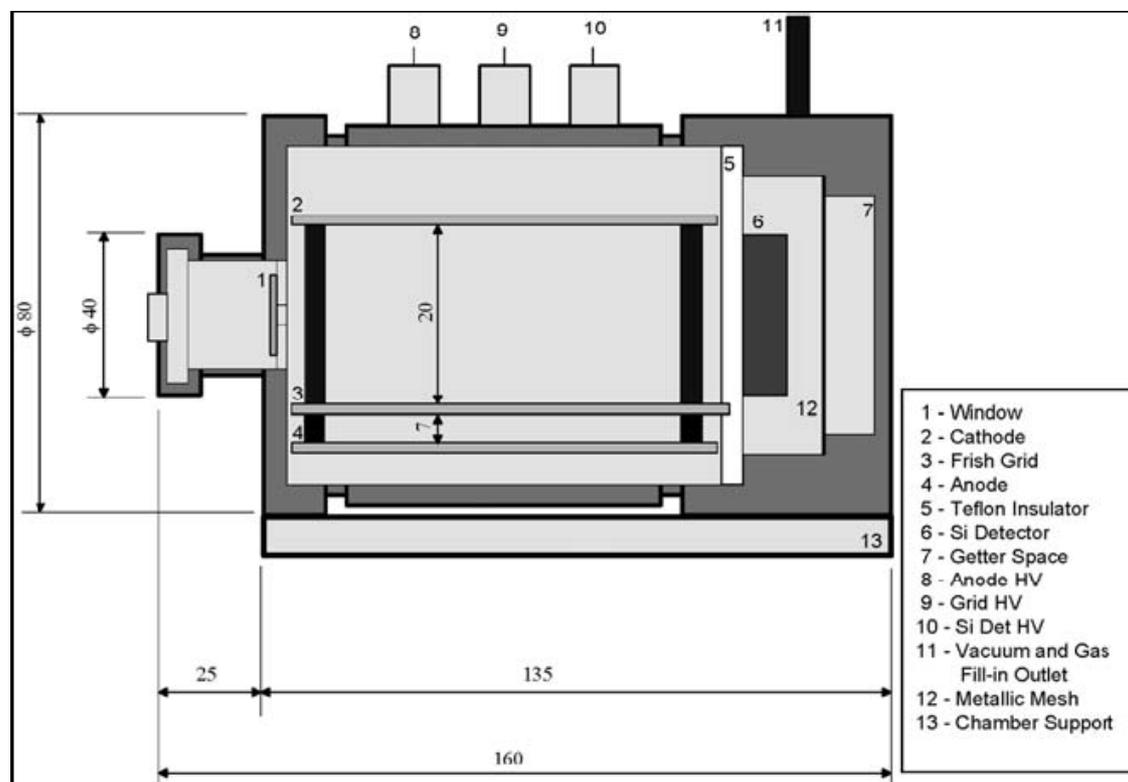
Fig. 1. The  $\Delta E - E_r$  telescope
