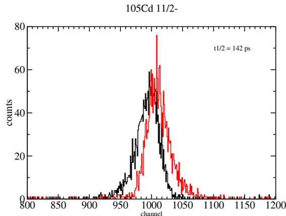
Figure 3: Time spectra for the  $11/2^-$  states in  $^{105}\text{Cd}$  [6]
