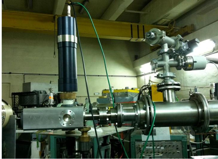
Fig. 4 : Irradiation cell for the time correlated single photon counting method. One can observe the photomultiplier (black cylinder) at the top of the irradiation cell.
