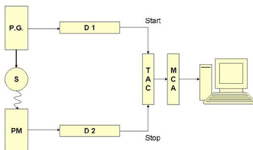
Fig. 1: Charged particles beam experiment : Block-diagram of time resolved fluorescence measurement apparatus (S : sample ; P.G. : pulse generator ; PM : photomultiplier (Hamamatsu R3235-01); D1 and D2 (ORTEC 584): discriminator 1 and 2 ; TAC : time-to-amplitude converter (TAC ORTEC 566) ; MCA : multichannel analyser).
