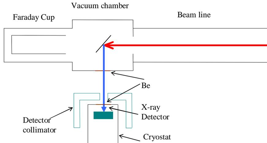
*Figure 3 Experimental setup for PIXE measurements schematics.*
