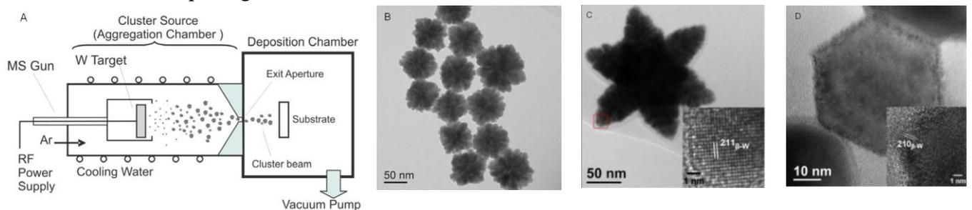
Fig.1: a) Schematic of the nanoparticle synthesis system; and TEM images of tungsten nanoparticles with different morphologies: nanoflowers (b), concave hexapodes (c) and faceted ones (d).
