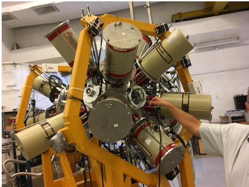
**Figure 1.** The Ge detector array of DFN Bucharest. We propose to replace the five forward Ge detectors by NE213 neutron detectors with special geometry.
