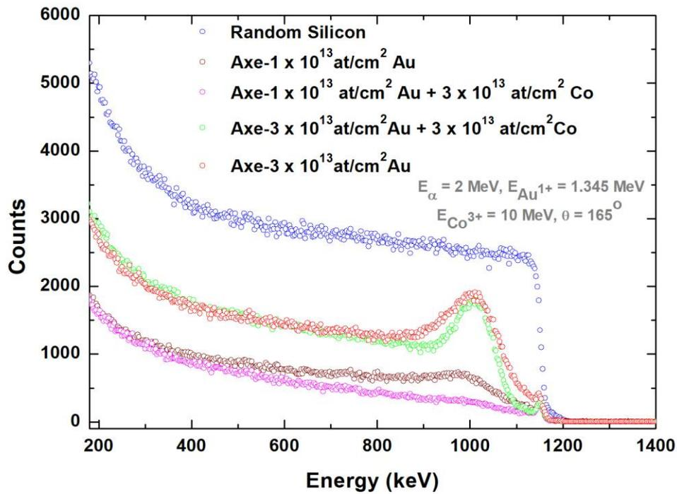
*Fig. 3: RBS spectra recorded in random and channeling orientations on Si crystals, implanted with 1.345 MeV Au<sup>1+</sup> ions, then irradiated with 10 MeV Co<sup>3+</sup> ions*
