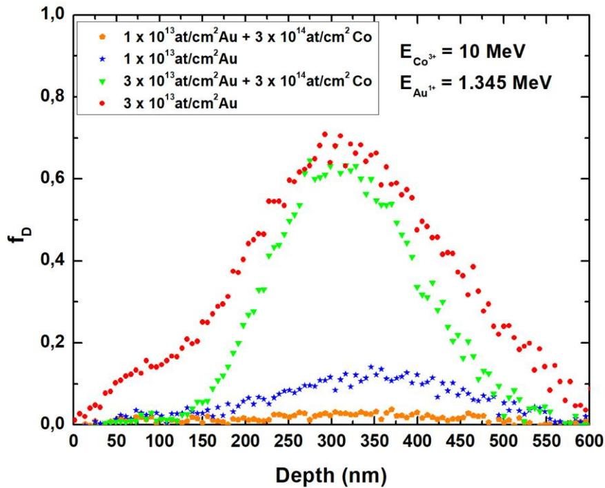
**Fig. 4:** Damage profiles in the Si crystals, implanted at RT with 1.345 MeV  $Au^{1+}$  ions and with 10 MeV  $Co^{3+}$  ions
