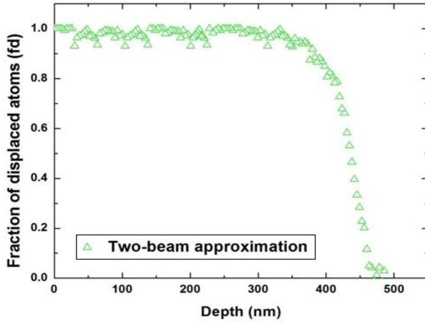
*Fig. 2: Depth distributions of the damage accumulated in a Si crystal, implanted at RT with 1.345 MeV Au ions at a fluence of  $1.25 \times 10^{15}$  at/cm<sup>2</sup>, extracted from the analysis of RBS/C spectra, using the TBA procedure*
