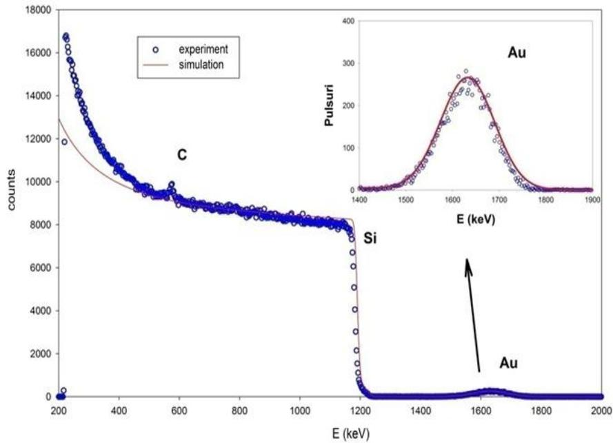
**Fig. 1:** 2 MeV  $^4\text{He}^{++}$  for 1.345 MeV Au-implanted Si (100) for Au -implanted specimens at  $1.25 \times 10^{15}$  at/cm<sup>2</sup>, collected charge was 264  $\mu\text{C}$ , with the detector at 165<sup>o</sup> and 145<sup>o</sup>
