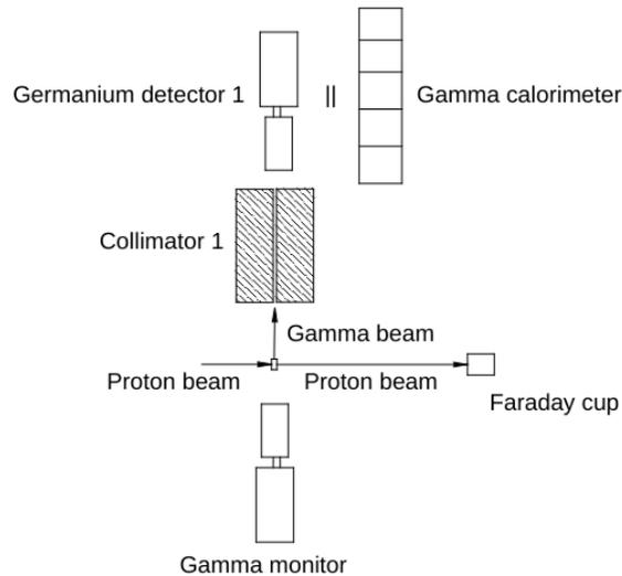
Figure 2: Experimental setup for calorimeter calibration
