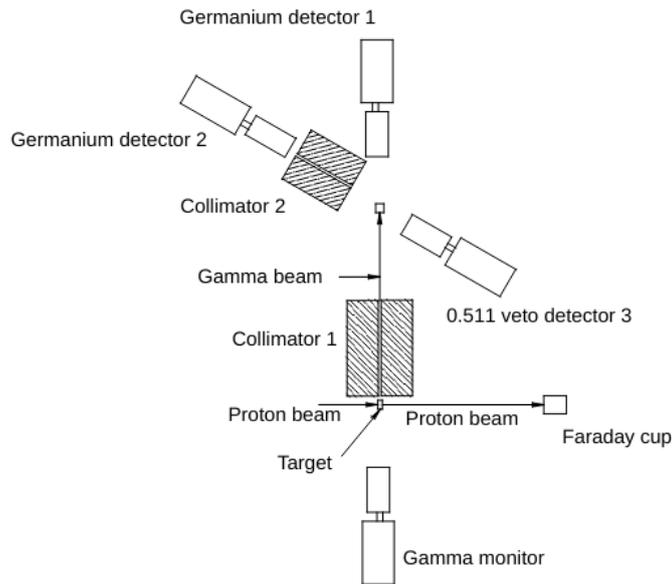
Figure 1: Effective Z determination setup
