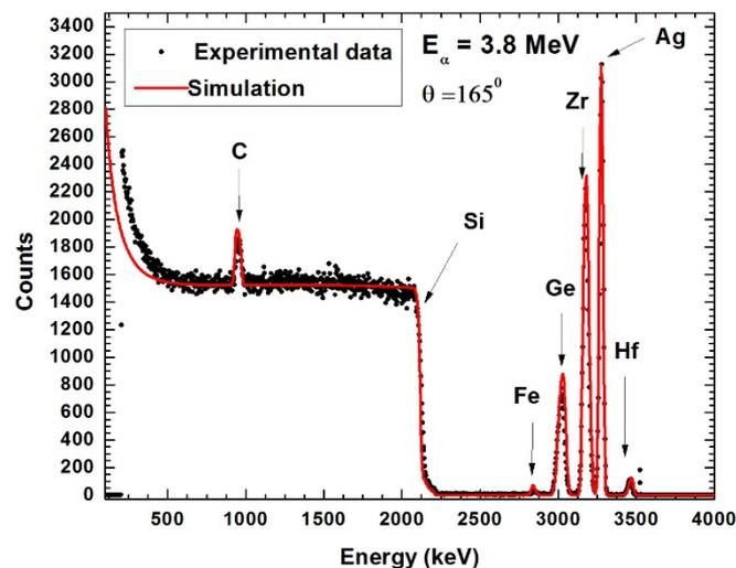
Fig. 1. RBS analysis of a thin ZrC film (200 nm) deposited on a SiGe/Si substrate; the SiGe layer is ~ 200 nm thick).
