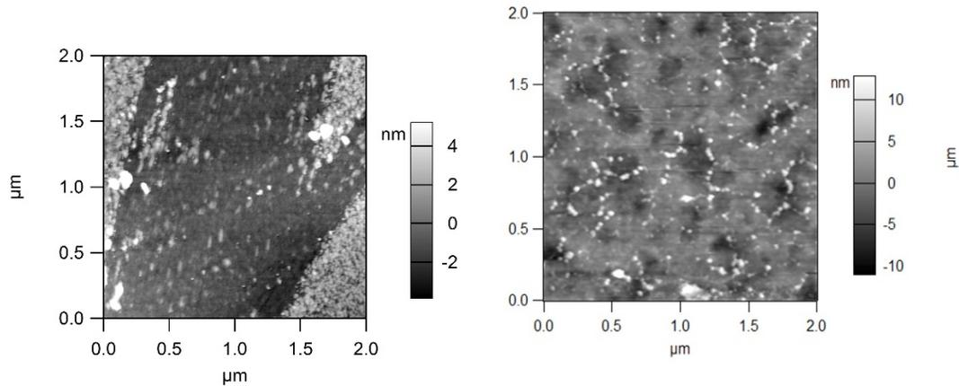
**Fig.1** AFM image of Si<sup>+</sup>/*n*-GaSb for as implanted sample (a) and after recovery treatment (b)
