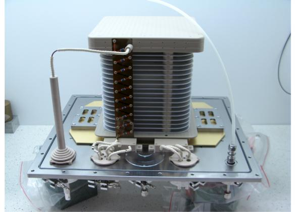
**Figure 2:** Upside-down view of the internal structure of the mini-eTPC detector, consisting of the drift cage, GEMs amplification stage, and the readout PCB (in yellow color).
