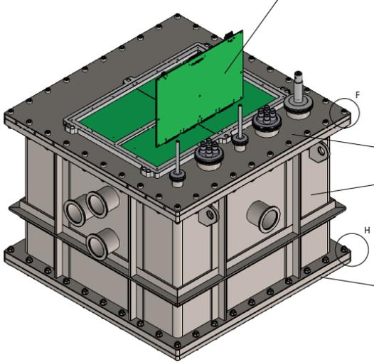
**Figure 1:** CAD design of the mini-eTPC detector reaction chamber in stainless steel. The gas stream inlet and outlet ports are located on the top end-cap cover. The standalone lateral port is the beam entrance point.
