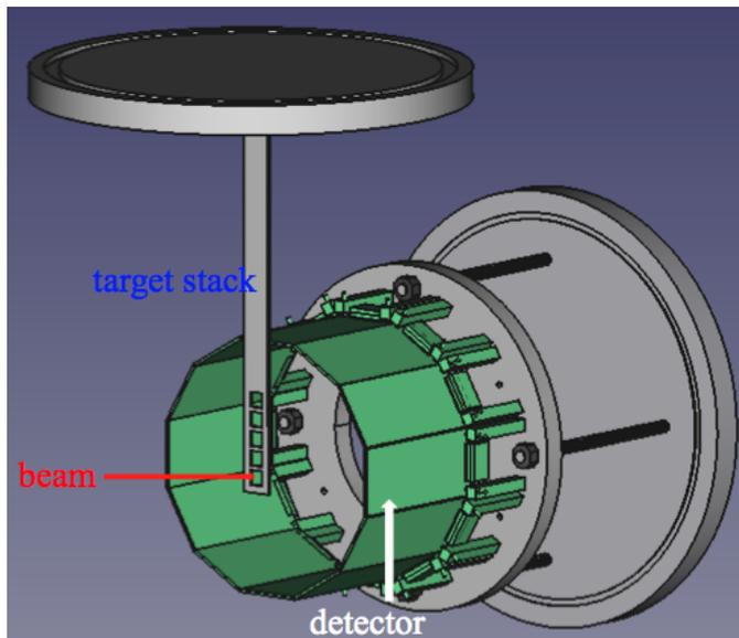
Figure 1: CAD simulation of the experimental setup inside the reaction chamber: twelve X3 silicon strip detectors in a cylindrical configuration, target ladder approximately 5 cm far from the center plane of the detectors.
